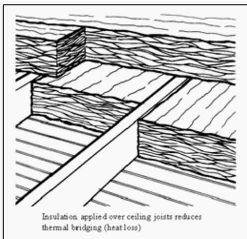
In addition to reducing energy use, increasing the insulation level in the structure between your ceiling and the roof ( attic space ) will keep your house warmer during the winter and cooler during the summer. Effective insulation and air sealing slow the movement of heat and air, and help prevent moisture accumulation in the attic.
